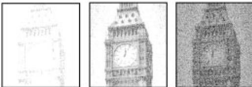
Figure 4. Images depicting the physical principle of ‘stochastic resonance’ and the effect that adding noise to a weak signal (left image) has on revealing an underlying signal (middle image), while adding too much noise (right image) can obscure the underlying signal. Figure adapted from Simonotto et al., 1997. Copyright 1997 American Physical Society
